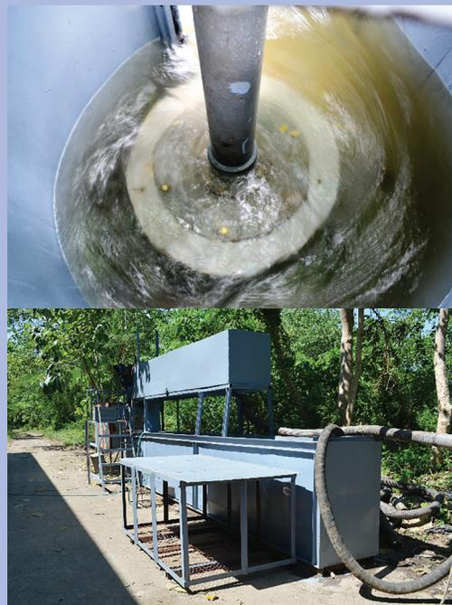
Turbine at work (top) and the Center's modified test rig (bottom)
