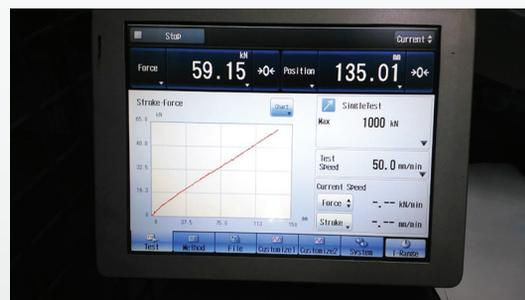
Actual conduct of 'Load vs Deflection' test for the HERT project.
