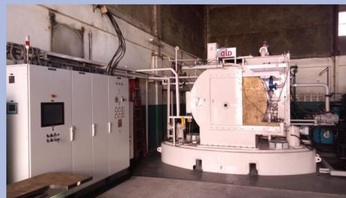
Vacuum Carburizing Oil-Quench Furnace
