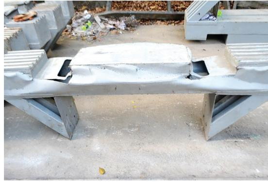
Impact Testing of an Anti-Climbing Mechanism
