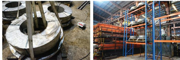
Weight of dummy weights determined using the load cell digital display (left), dummy weights are used to provide full load on steel racks (right).
