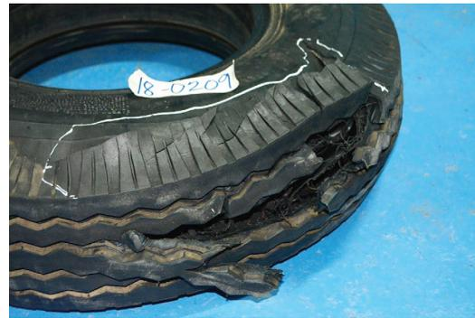
Fractured sample of a tire subjected to load/speed and endurance test.
