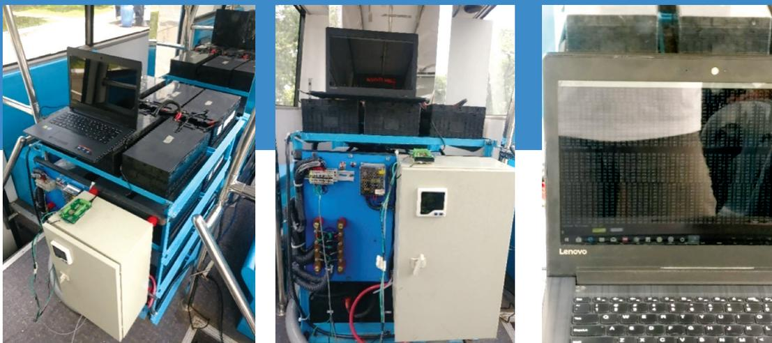
(Left and center) Set-up of the battery management system (BMS) showing the newly-installed lithium ion batteries; (right) laptop displaying the output of the BMS.
