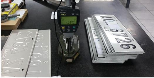
MIRDC conducts dimensional inspection of motor vehicle license plates.
