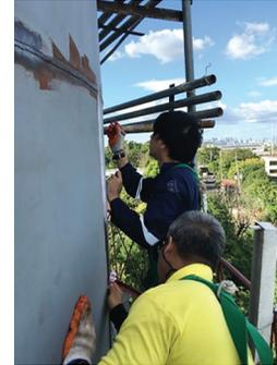
The NDT team conducts Liquid Penetrant testing of the overhead water tank of the MIRDC.
