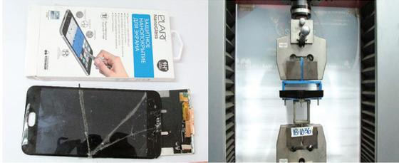
Glass cellphone screen undergoes micro Vickers hardness test (left); Bag Ring Comp is subjected to a breaking load test (right).
