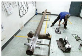
Drill rods of the Maynilad water system projects undergo Magnetic Particle Testing (left), and Visible Magnetic Particle testing is conducted to ensure quality of welding (right).
